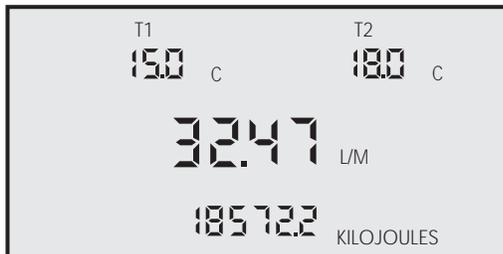
Display shows flow in LPM or GPM, t1 temperature, t2 temperature, and heat units in Metric or English Units.
