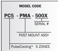
Post Mount Ass'y 5 Zone Cooling Valve Ass'y Model: PMA-500X \$3,200.00 Shown with 1" Supply / Return 2(3/8") to and from Mold Conn 2(3/8") to and from Mold Conn 1/2" to and from Mold Conn 1/2" to and from Mold Conn 3/4" to and from Mold Conn
